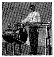
Bird Pressure Filters are built in a wide range of sizes up to 1500 sq. ft. of filter area. You can use this pilot-size Bird Pressure Filter for preperformance testing. Say the word and we'll arrange for it.
